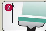
Apply first coat from bottom to top direction with a putty blade.
